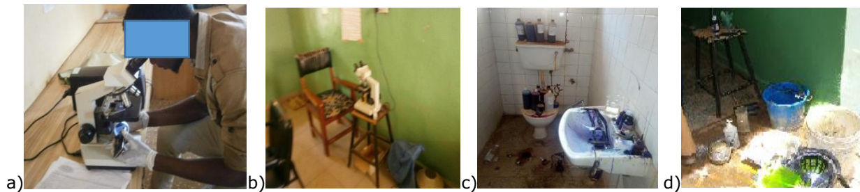
Fig 6 showing; (a) a technician examining a slide using touch light of a mobile phone as source of light to the microscope; (b) microscope kept on a chair, (c) toilet used as staining basin due to lack of a staining rack, and (d) staining for malaria parasites done outside the laboratory
