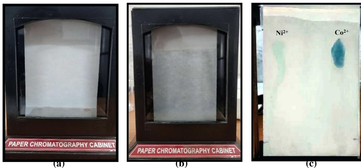
Figure 3. \text{Ni}^{2+} and \text{Co}^{2+} separation using paper chromatography by 4% \text{NH}_4\text{OH} solution
