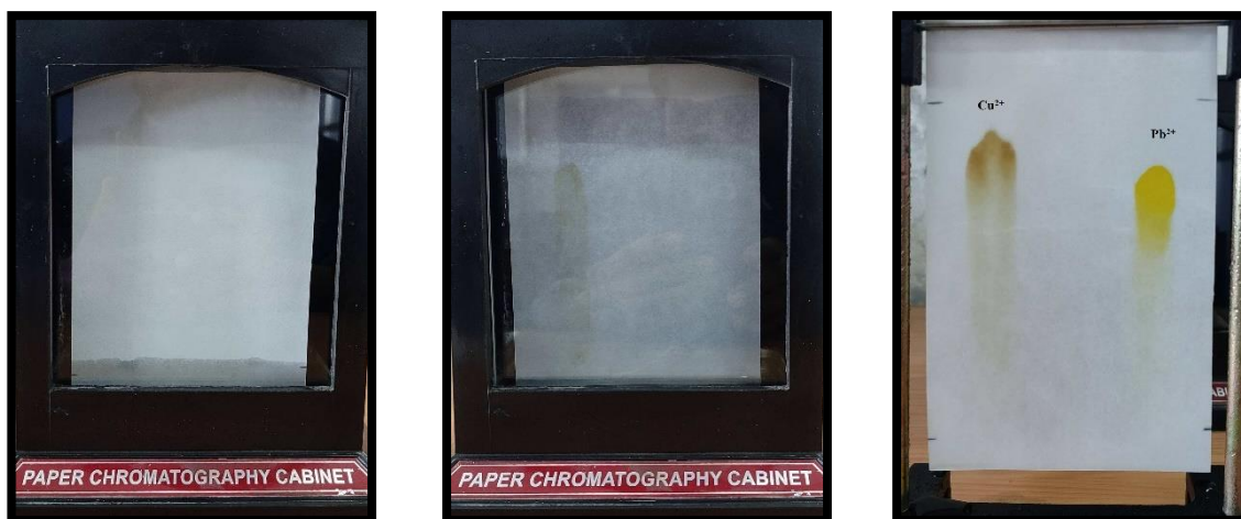
Figure 2. \text{Cu}^{2+} and \text{Pb}^{2+} separation using paper chromatography by 1% KI solution
