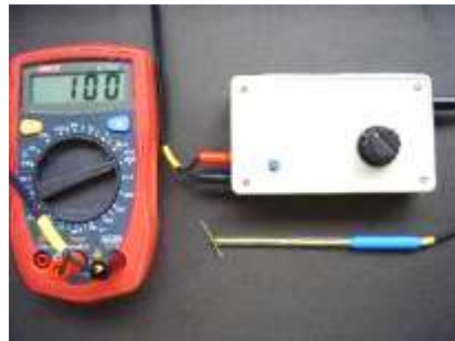
(Fig. 2) Experimental setup for setting full scale by short-circuiting the probe with a thread of metal wire
