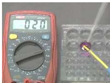
(Fig. 26) Conductivity measurement during titration
