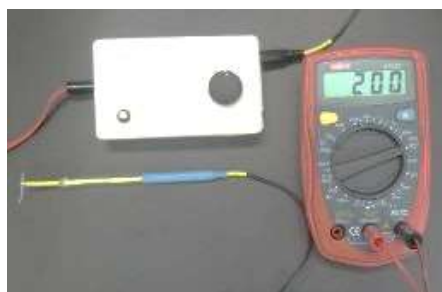
(Fig. 25) Calibrate the sensor by adjusting to 200 mV
