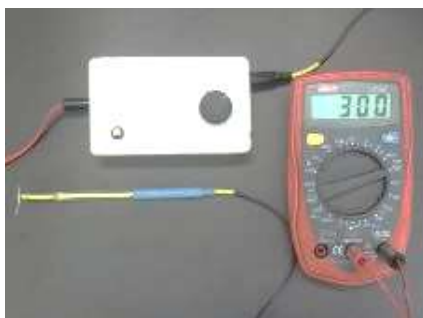
(Fig. 22) Full Scale adjustment at 300 mV
