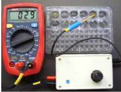
(Fig. 3) A testing solution showing 29/100 conductivity
