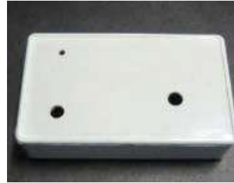
(Fig. 16) Utility box with drilled holes of various sizes
