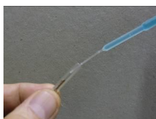
Fig. 1 Use a micro-tip plastic pipette to fill the small chamber with 1M CuSO 4 solution
