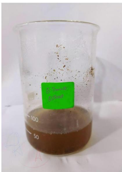
Figure 2: The color change noticed to dark brown after the reaction with the sodium selenite solution
