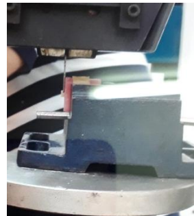
Figure 2: The specimen has been secured in a universal testing machine (Laryee, China)
