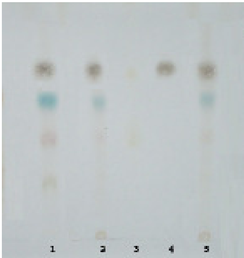
Figure 1. TLC of F. gardenia . 1, Sample of Tangkening granule; 2, reference material of F. gardeniae ; 3, negative sample without F. gardeniae ; 4, reference compound of geniposide; 5, material of F. gardenia .
