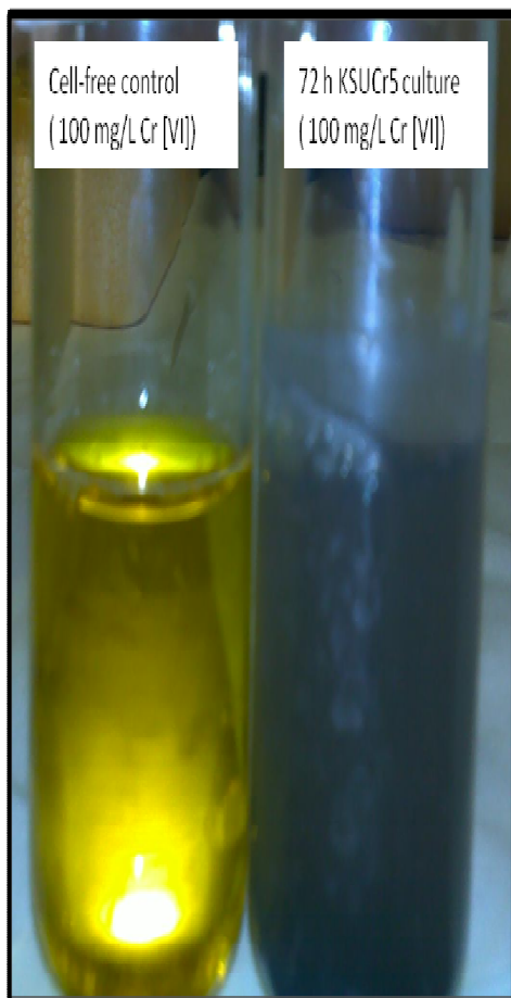
Figure 2. Chromium reduction by Bacillus sp. KSUCr5. The strain was grown in alkaline medium containing The strain was grown in alkaline medium containing 1% Na 2 CO 3 , 10% NaCl, 1% glucose and with chromium concentration of 100 mg/L and incubated for 24 h at and incubated for 24 h at 30°C with shaking (150 rpm). Complete Cr(VI) reduction was achieved within 72 h and white-grayish precipitate visible at the bottom of the bottle (Right). Cell-free control was used to monitor any abiotic Cr(VI)-reduction (Left).
