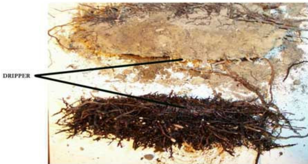
Figure 3. Root density around the emitter opening in SDI system.
