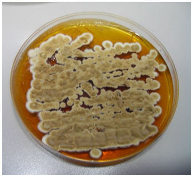
Figure 6. Visual fungal growth on LDPE/potato starch blend after 84 days incubation.
