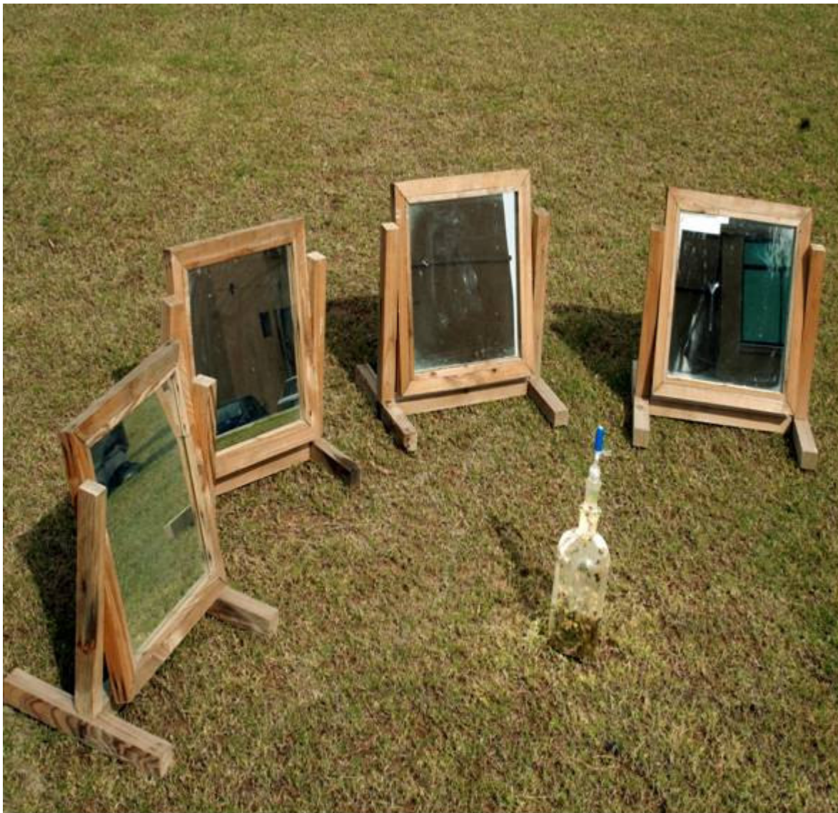
Figure 8. Apparatus for photo catalysis of water hyacinth.
