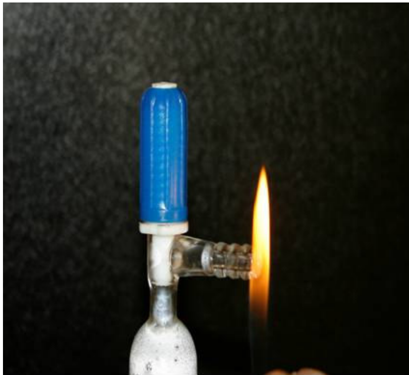
Figure 9. Burning of photo catalytically produced methane.
