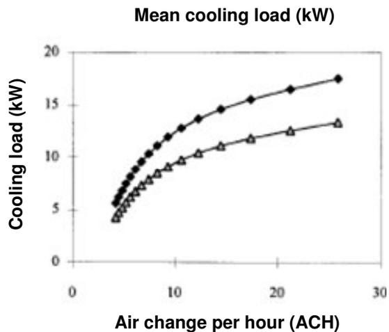
Figure 7. Cooling load by night ventilation for desired room indoor air temperatures of 23 and 25°C.
