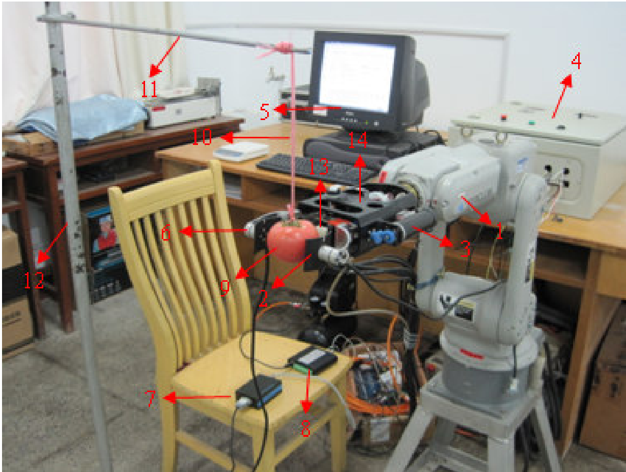
Figure 1. Experimental system. 1: tomato-harvesting robot; 2: finger; 3: motor; 4: control cabinet; 5: computer; 6: pressure sensor; 7: signal amplifier; 8: USB5935 data acquisition instrument; 9: tomato; 10: string; 11: beam; 12: height-adjustable stand 13: sucker; 14: end-effector.
