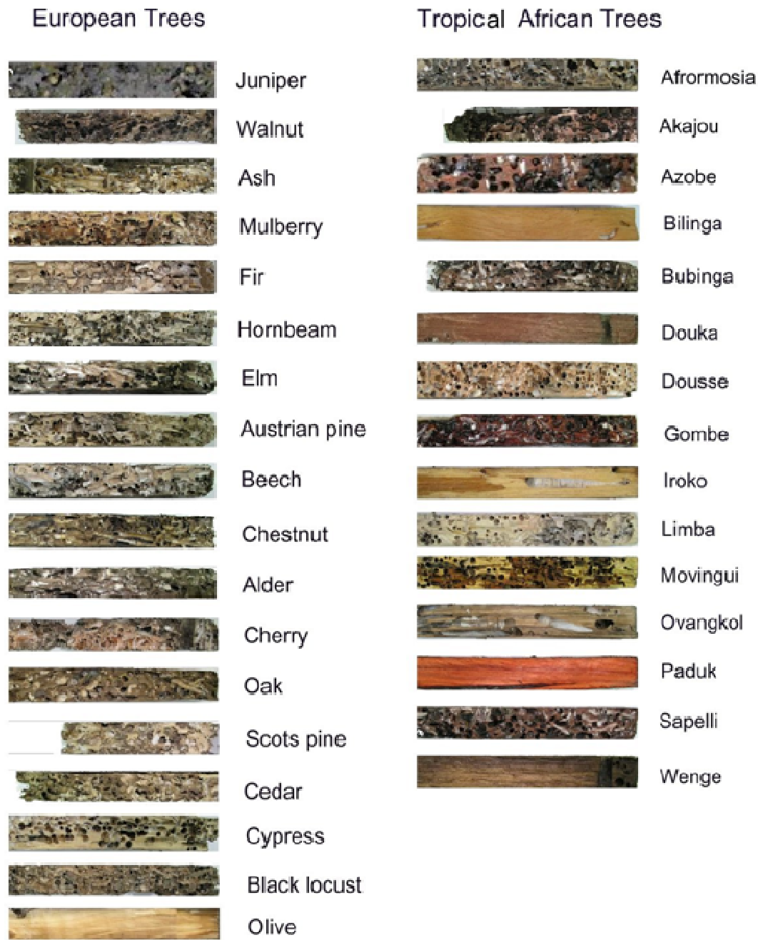
Figure 2. The samples from Iskenderun harbour where the highest degradation after exposure time for 1 year.
