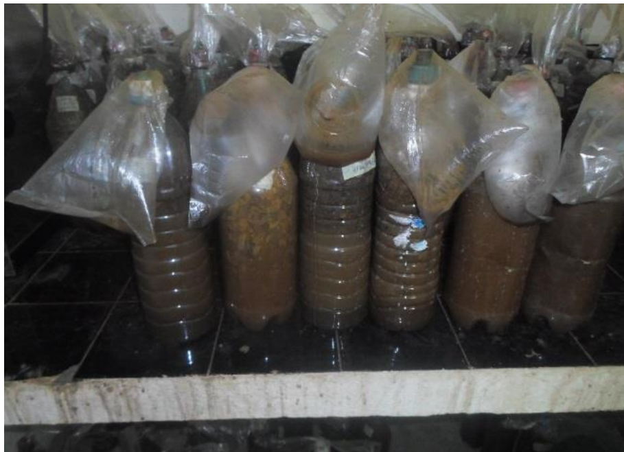
Figure 1. Mini-bioreactors producing biogas from dead neem leaves.
