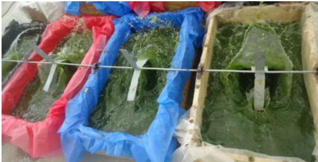
Figure 3. Aeration by modified rotating paddle wheel.
