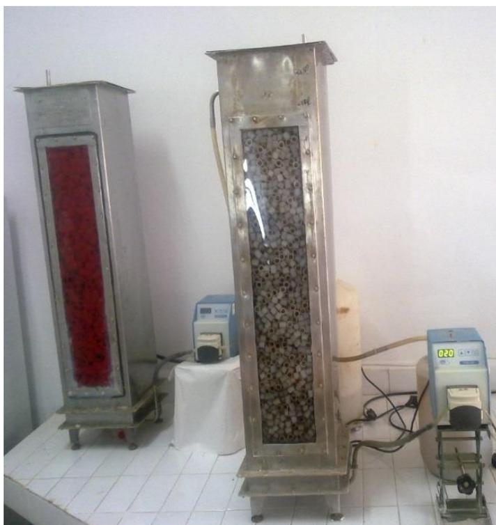
**Figure 3.** Experimental anaerobic bioreactor system.
