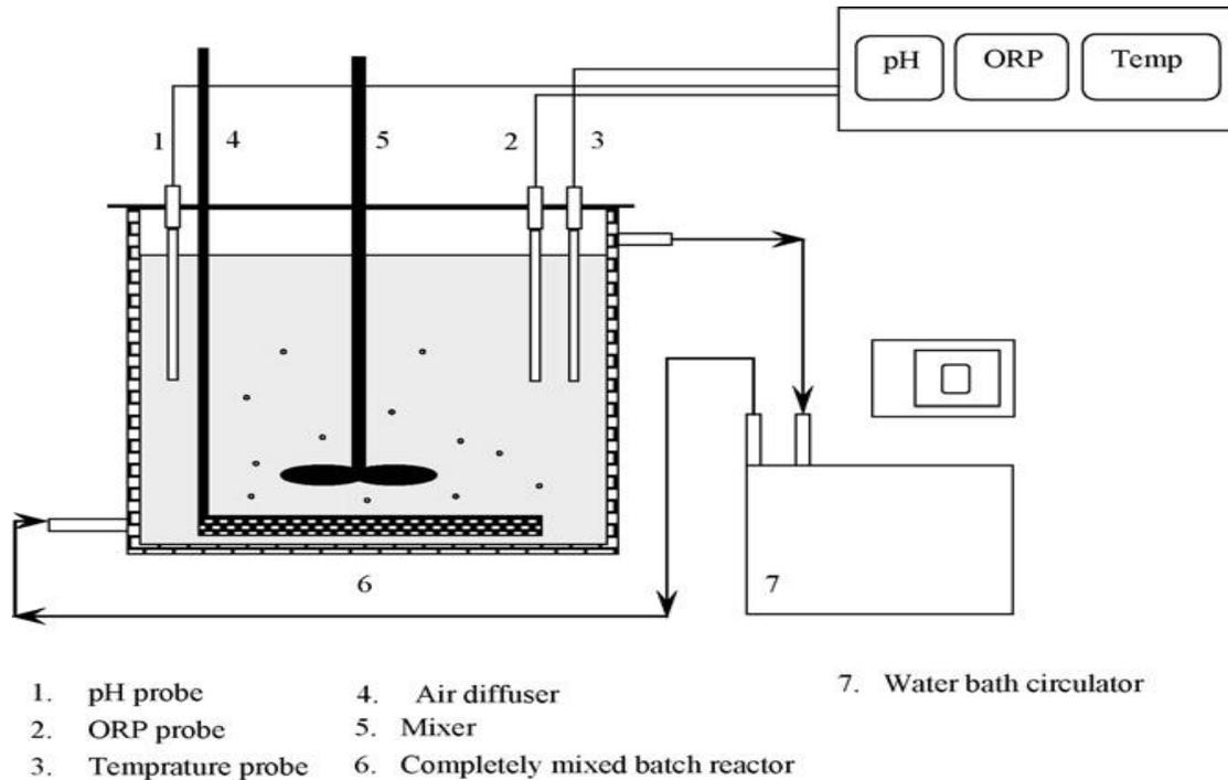
Figure 1. Schematic diagram of bioleaching experiments.
