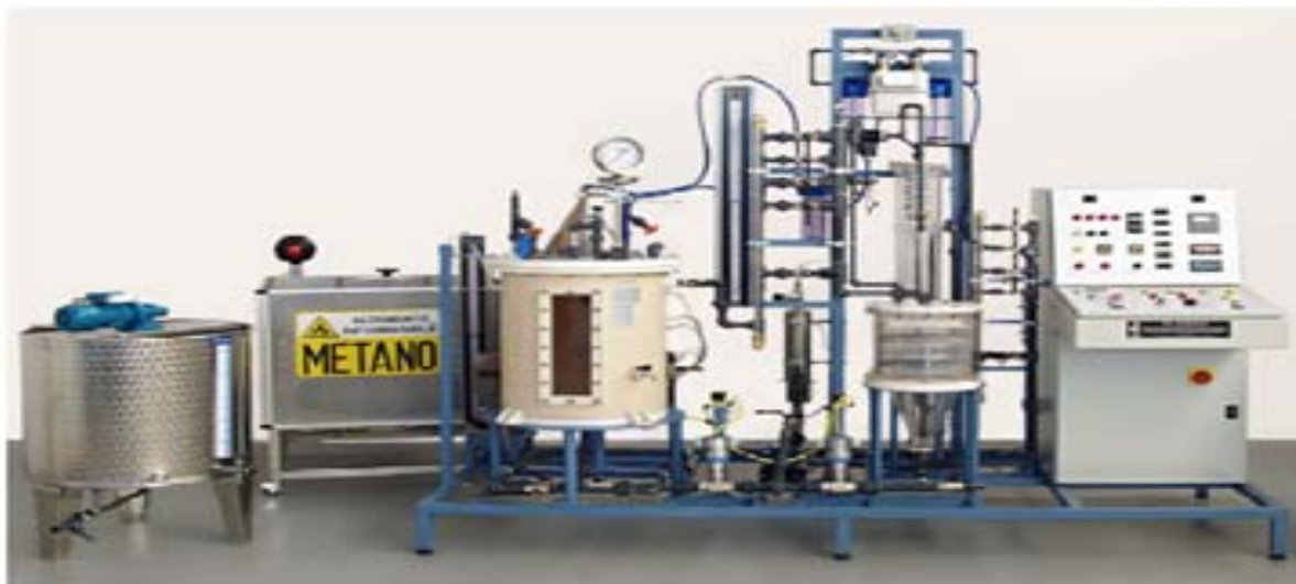
Figure 1. RE-BIOMAS-pilot plant for the production of biogas from biomass.
