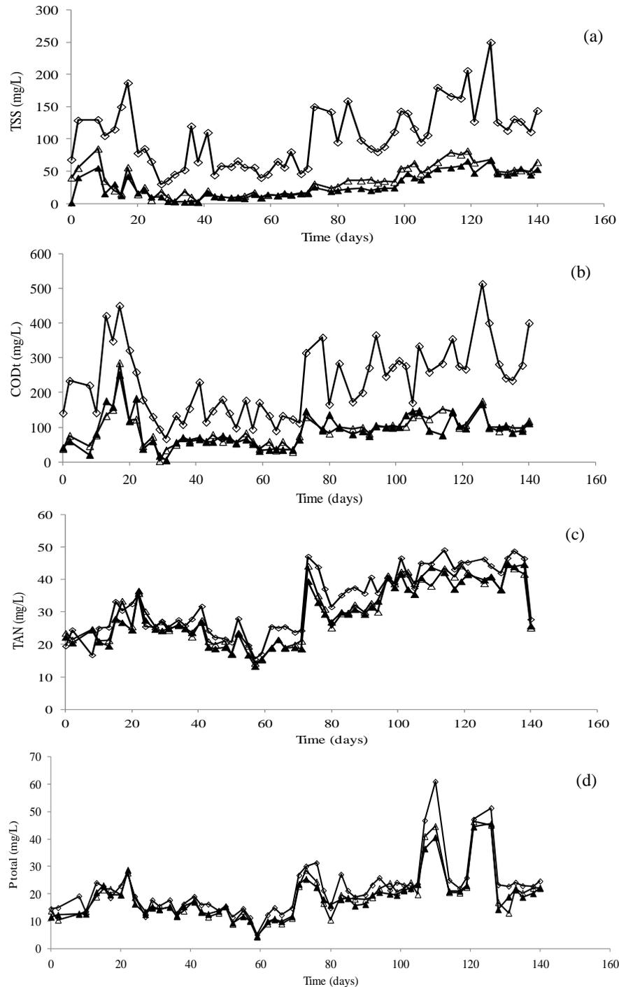
**Figure 5.** Concentrations of (a) the total suspended solids (TSS), (b) the total chemical oxygen demand (COD<sub>t</sub>), (c) the total Ammonium nitrogen (TAN) and (d) the total phosphorous (P<sub>total</sub>) in the Influent (◇), ACF1 Effluent (△) and ACF2 Effluent (▲) during the entire study period.
