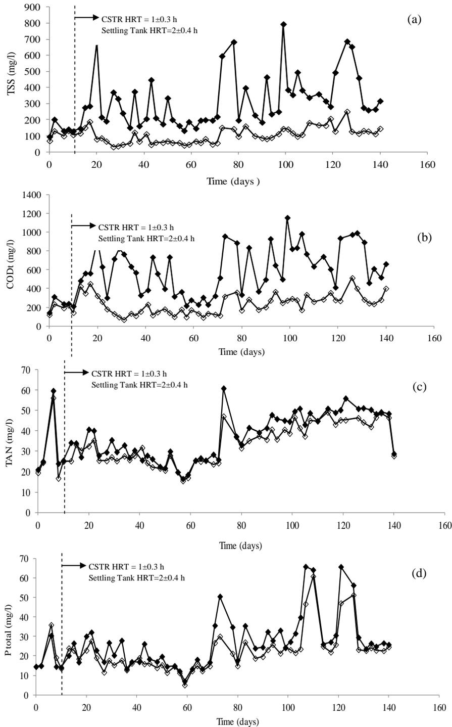
**Figure 4.** Influent (◆) and effluent (◇) concentrations of (a) the total suspended solids (TSS), (b) the total chemical oxygen demand (COD<sub>t</sub>), (c) the total Ammonium nitrogen (TAN) and (d) the total phosphorous (P<sub>total</sub>), in the high rate activated sludge system during the entire study period.
