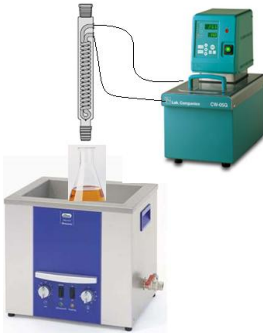
Figure 1. Sono-reactor for pre-treatment of CPO.
