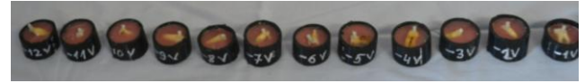
Figure 4. Appearance of some samples from the control group ( G_{\text{control}} ) prepared for the microshear bond strength tests.
