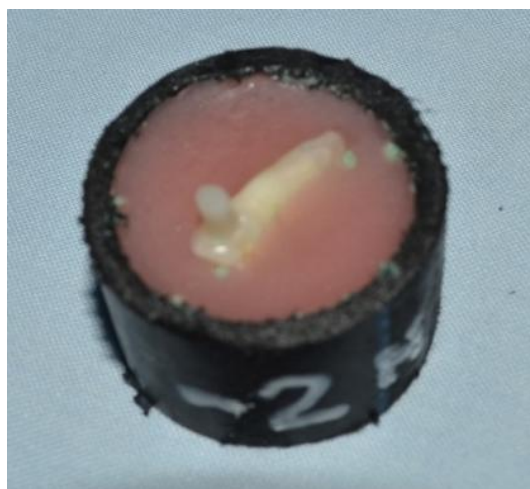
Figure 3. Appearance of a tooth with cylindrical restoration from composite resin fixed for microshear bond strength test.
