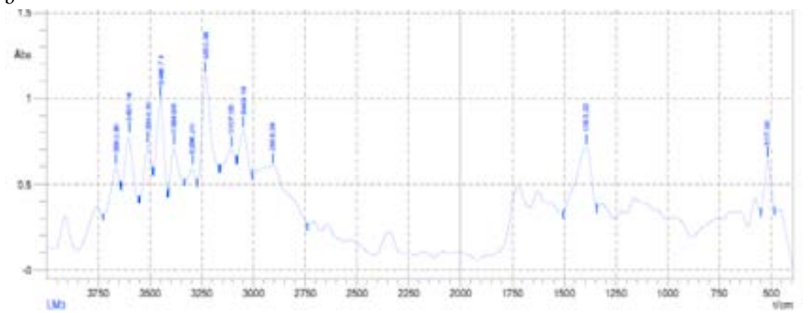
Figure 3: Fourier transform infra-red (FT-IR) spectrum of (a) lipid matrix based on beeswax and Phospholipon® 90H (P90H) (LM 1 ), (b) caprol-PGE 860 and (c) Phospholipid-modified beeswax-based lipid matrix structured with caprol-PGE 860 (LM 3 ).
