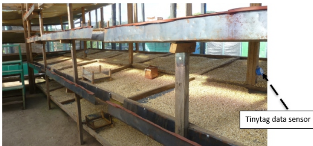
Figure 3: Location of temperature and relative humidity sensors at the 2 nd layer in dryer
