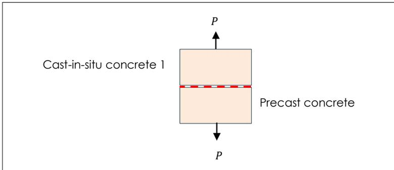
Figure 2: Cross section of interfacial tensile bond specimen
