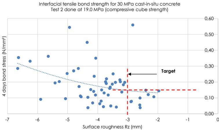
Figure 7: Interfacial tensile bond strength at four days for 30 MPa concrete
