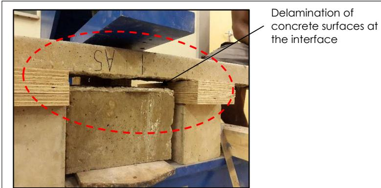
Figure 5: Precast and cast-in-situ concrete delaminates
