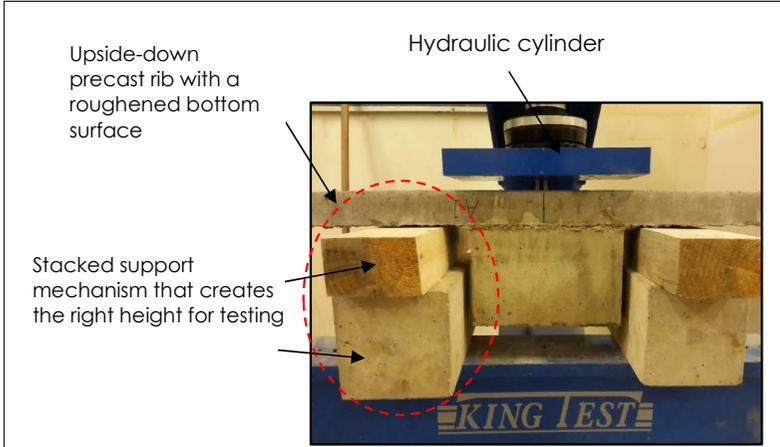
Figure 3: Placement of the specimen into the beam press apparatus
