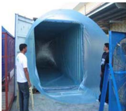
Figure 5. TranSafeliner™ being installed in a standard shipping container, 2008.
