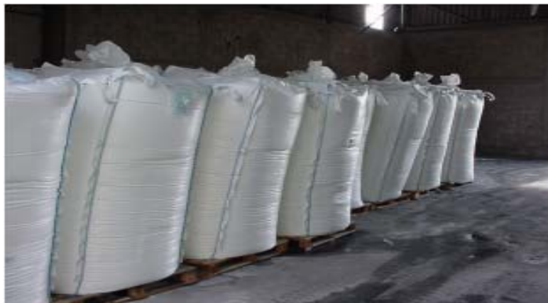
Figure 4. One tonne SuperGrainbags-HC™ storing paddy with woven inside protective polypropylene bag.
