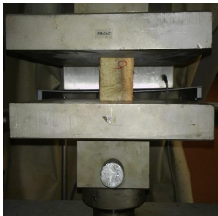
Figure 5: Arrangement and failure mode of compression perpendicular
