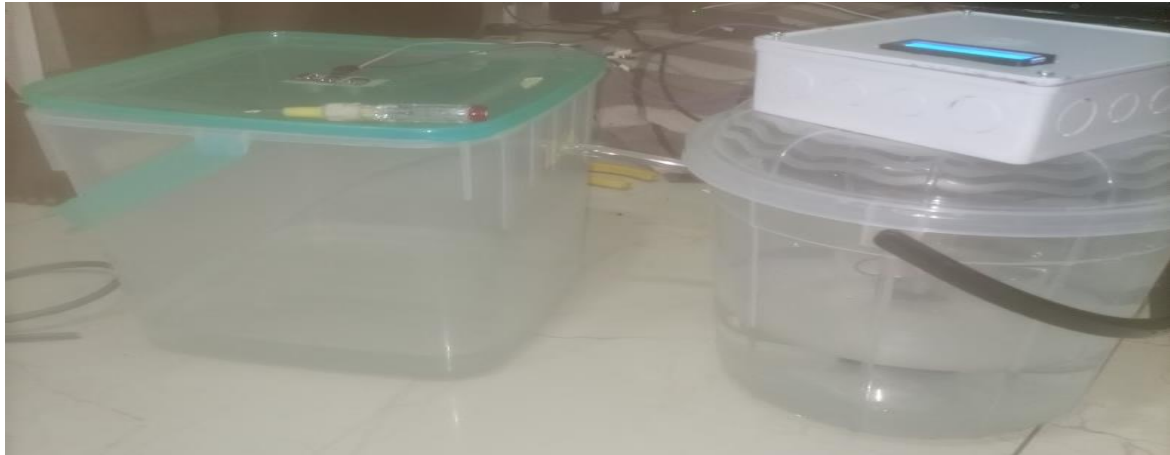
Figure 9: Image of the sections of the system (constructed device, water tank and bore-hole representation)
