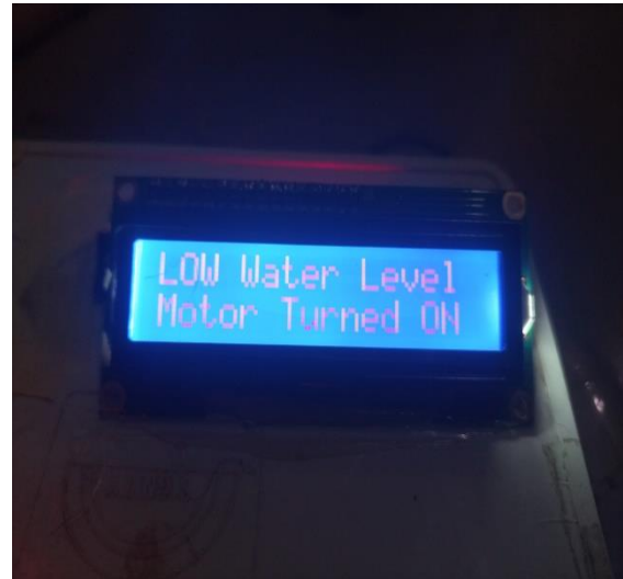
Figure 11: Displayed image of when the tank is low
