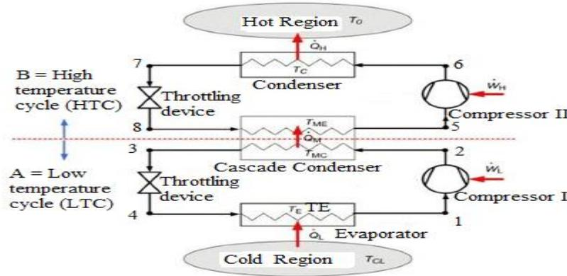
Figure 1: A two-stage cascade refrigeration [5]
