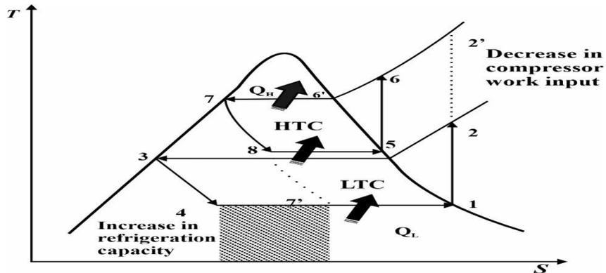
Figure 6: T-S diagram for actual two-stage vapour compression cascade cycle
