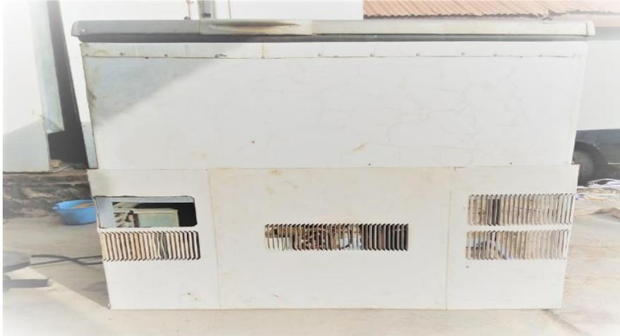
Figure 5: Cascade refrigeration machine
