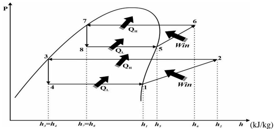
Figure 7: P-h diagram for two-stage vapour-compression refrigeration cycle
