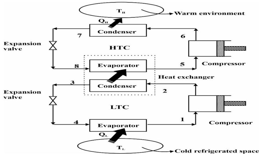
Figure 3: The schematic diagram of the two-stage cascade refrigeration system
