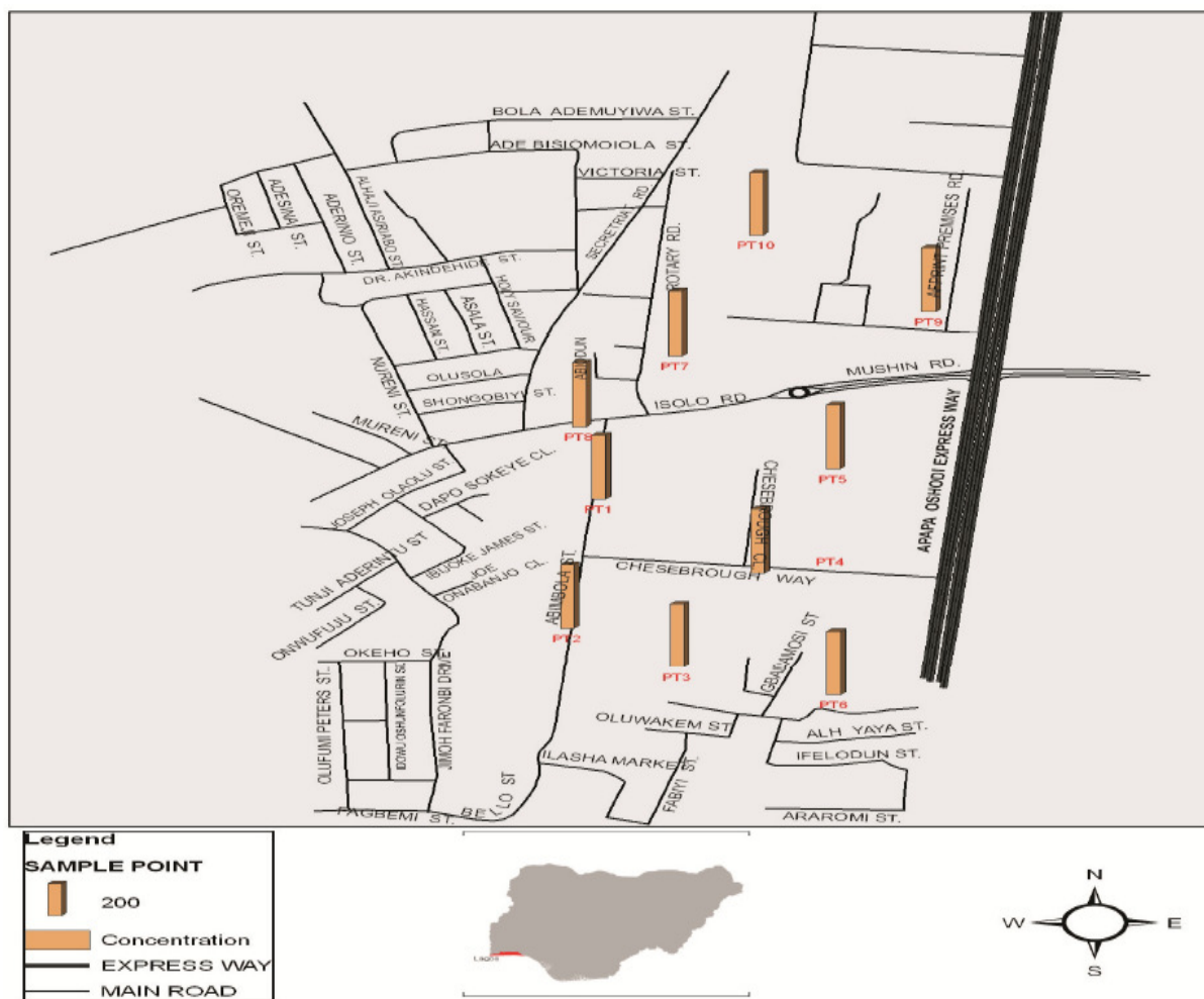
Figure 3 GIS Base - Map of Isolo Industrial Area Showing Spatial Distribution of Total VOCs Concentrations.
